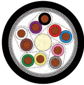
Marking for 3909696: SAB BRÖCKSKES · D-VIERSEN · Special Cable 5x2x0.50mm 2 3909696 CE
